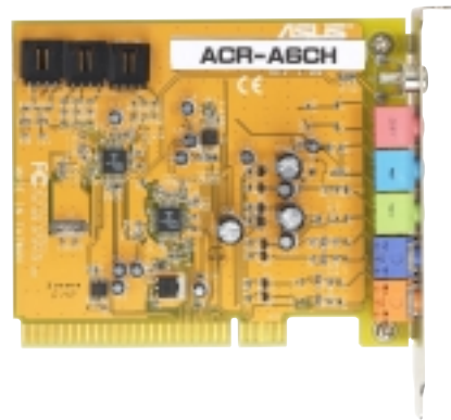
A7N266-E Advanced Communication Riser (ACR)
