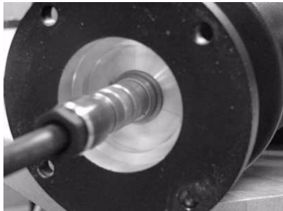
Figure 3.7 Composite cable connected to MIC612 camera
