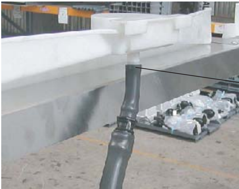
Typical hose connection to Water Spreaders Inlet. 8 places.
