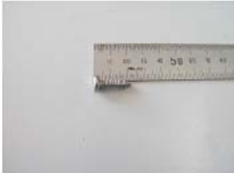
Screw 19x5mm Phlp. SS. P/No 9610013
