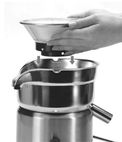
STEP 2. Align the arrows on the Stainless Steel Filter Basket with the arrows on the Motor Drive coupling and push down until it clicks into place. Ensure the Stainless Steel Filter Basket is fitted securely inside the Filter Bowl Surround and onto the Motor Base.
