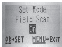
[Step 1] -set Field Scan Mode to “On”
