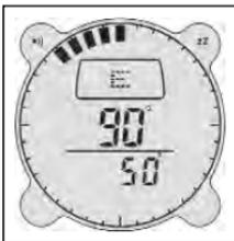
To operate the compass in Homing Mode go into the Compass Mode first, then press **MODE** button to get into Homing Mode.
