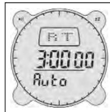
To set the Countdown Timer press and hold down the **ADJ** button for 3 seconds, which will cause the seconds setting to blink. Adjust with the **UP** or **DOWN** button, and then press the **MODE** button to adjust next setting. Press the **ADJ** button to save settings and exit. Press the **COMP** for 'AUTO' to allow Countdown Timer to repeat function automatically, and press **COMP** again to turn off 'AUTO' function.
