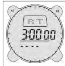
Press any button when alarm sounds to stop the Countdown Timer. If nothing is pressed the Countdown Timer will stop beeping after 10 seconds, but it will continue if the 'AUTO' function is set on. To stop the Countdown Timer if the 'Auto' function is on, you must go to the Countdown Timer Mode and press **COMP** to turn off the 'Auto' function and then press **UP** button to stop it.
