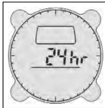
For 24/12 hour setting press **MODE** button until Time Mode is displayed. Press and hold down **ADJ** for 3 seconds. Press **MODE** button and scroll through settings until 24/12 hour setting appears, then press **UP** or **DOWN** button to enter desired setting. Press **ADJ** button at any time to save changes and exit.
