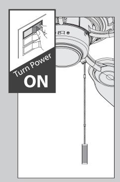
The pull chain controls the fan: from high to off.
