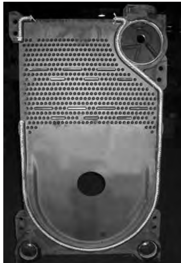
Figure 7: Affixing the Fiberglass Rope
