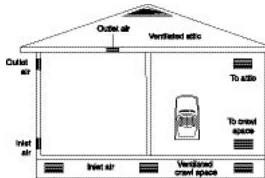
Fig.3 Ventilation Air From Outdoors
