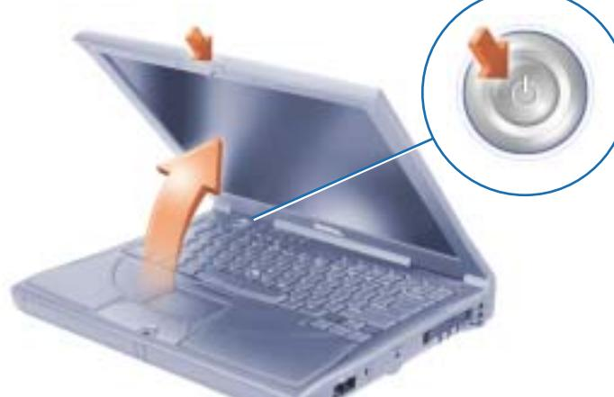
Open the display, and press the power button to turn on the computer. Follow the prompts on the screen to complete the operating system setup.
