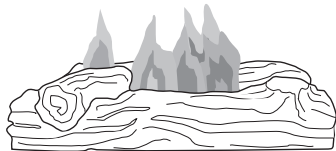
Figure 54 - Incorrect Burner Flame Pattern
