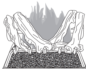
Figure 40 - Typical Flame Pattern
