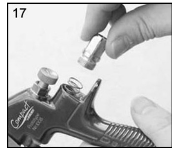
17. Replace Valve Spring and screw in Housing (10).
