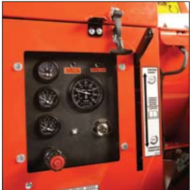
ECHO Bear Cat's hand-operated manual engagement lever assures ease of use.
