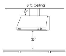
8 ft. ceilings: When the hood is installed 30" above the cooking surface and there is no soffit or upper cabinetry, order one 12" duct cover accessory.
