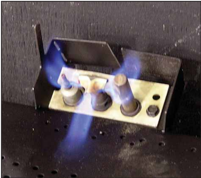
Figure 3.2 Standing Pilot Flame Patterns
