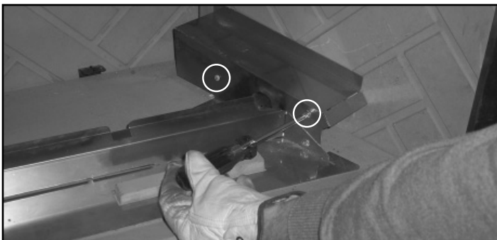
Figure 6.2 Remove Pilot Shield
