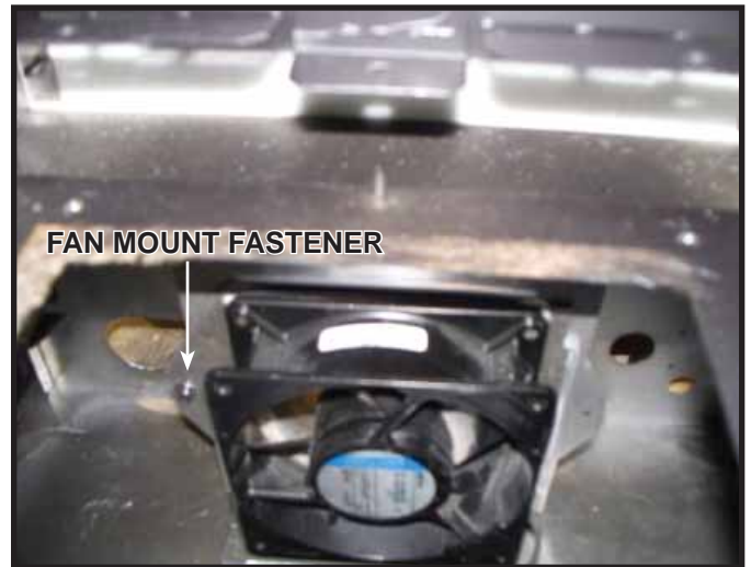
Figure 12.14. Fan Mount Fastener Location.
