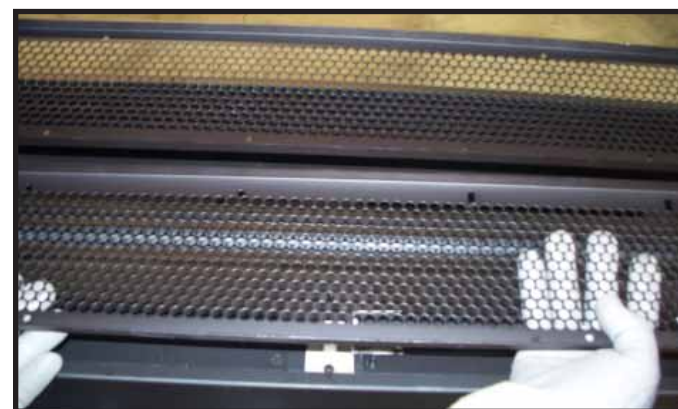
Figure 12.10 Lifting Base Pan Up and Out.
