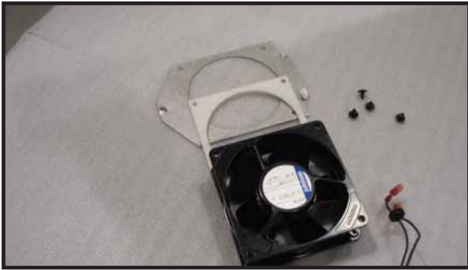
Figure 12.17. Remove Mounting Plate
