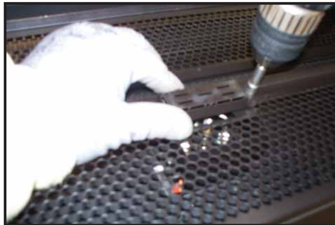
Figure 12.8 Removing Pilot Shield
