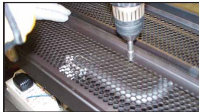
Figure 12.9 Removing Screws from Base Pan.
