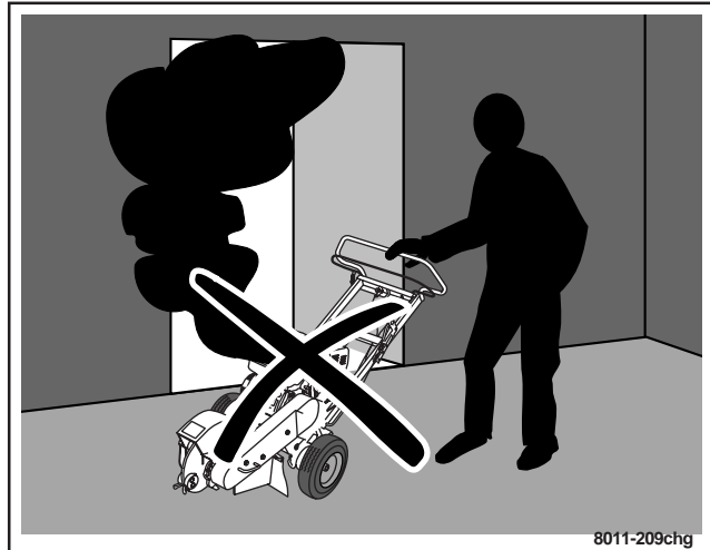
The engine exhaust is poisonous. Never run the engine indoors.
